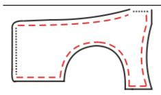
Follow vehicle manufacturer's replacement procedures to prepare the service panel for replacement. Follow vehicle manufacturer's replacement procedures for welding the joint between the rear body and the quarter panel, as well as the sail panel. Adhesive can be used on all other areas, lower panel, wheel opening, door jamb, and trunk drip rail. Follow directions for surface preparation and applying adhesive.
