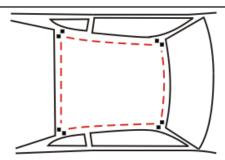
Follow vehicle manufacturer's replacement procedures to prepare the service panel for replacement. Leave a space of two inches at each of the four corners to allow for two plug welds or a two inch lap weld. Use adhesive around entire perimeter of the roof and on the roof bows if applicable. Follow directions for surface preparation and applying adhesive. NOTE: On extended length van roof panels, 2 - 3 extra plug welds should be placed evenly in each side of the roof panel.
